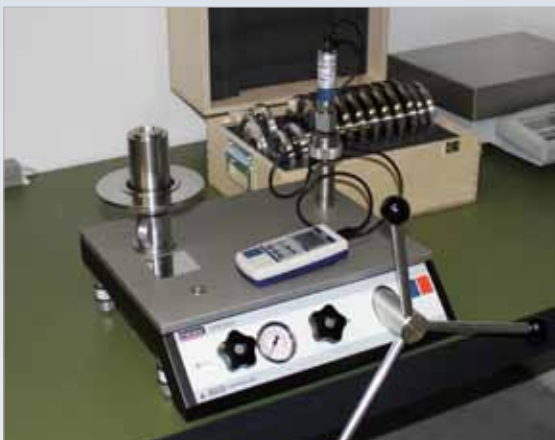
Piston manometer for calibration of various test specimens.
