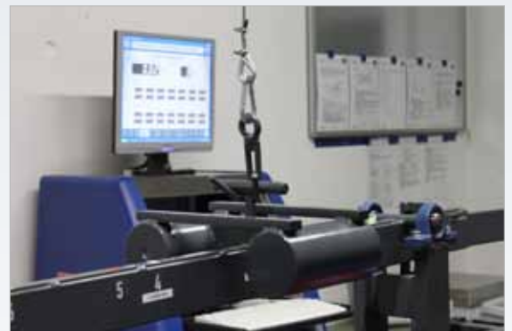
Calibration weight placed on calibration device
